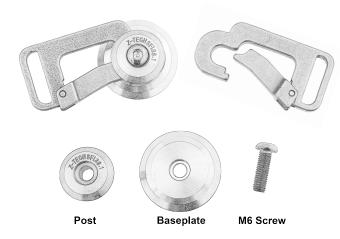
Remove black cap from back of Helmet Kit before installing. Set the Baseplate (pictured above) against helmet shell centered to the M6 insert. Then put the M6 Screw through the Post with thread lock-tite "blue" on the end of the screw. Align the Post and M6 Screw through the Baseplate and carefully tighten the M6 Screw into the helmet without cross-threading during installation. Tighten snuggly and allow thread lock-tite to dry.
