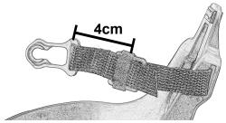
(diag. 1a: 4cm between end of clip and center of H buckle)
